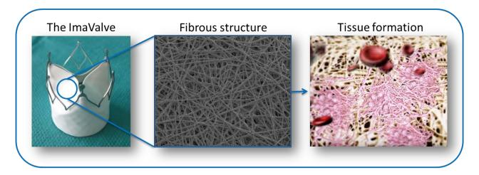
**Form follows function**: This image shows a heart valve prosthesis, for non-invasive surgery, made of a bio-resorbable supramolecular polymer. The polymer has been designed and processed in a way to mimic the architecture of the heart valve on microscopic and macroscopic levels. This way, it provides the ideal scaffold that more accurately recapitulates its function. The magnification reveals the fibrous structure that promotes cell-ingrowth and induces tissue formation.
